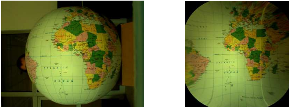
Example of remapping of a spherical object using CreateSphereMap and RemapImage . Image before and after remapping.
