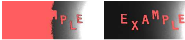
Results of ThresholdToRegion and ThresholdToRegion_Dynamic on images with uneven light.
